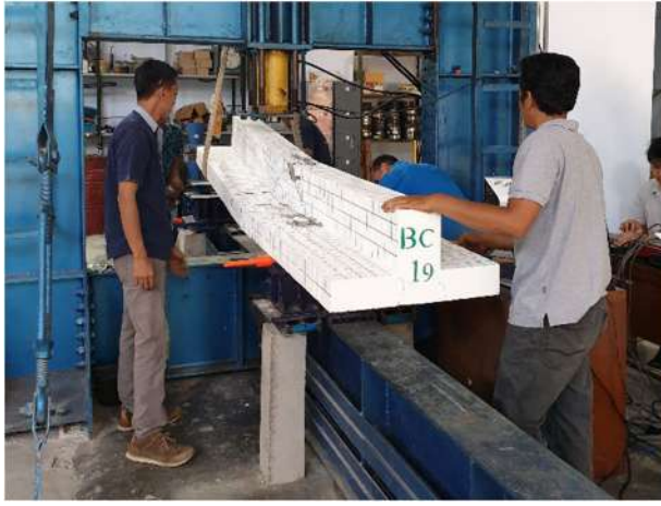
Figure 4. RC T-beam after the tests.
