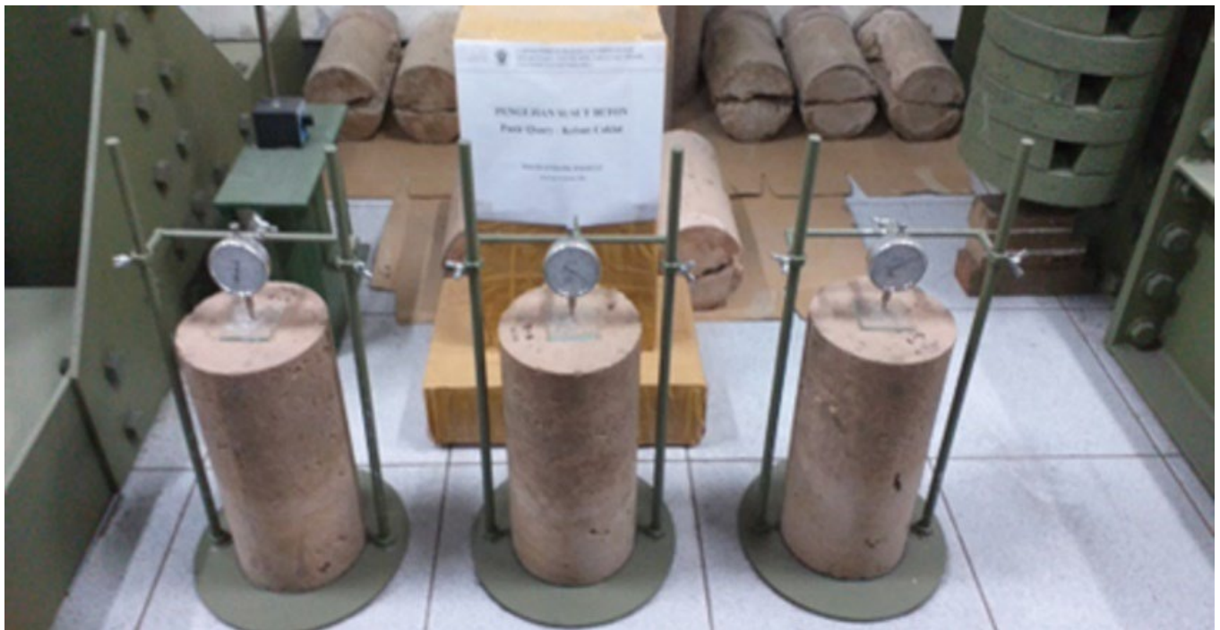
Figure 2. The measurement of shrinkage deformation.
