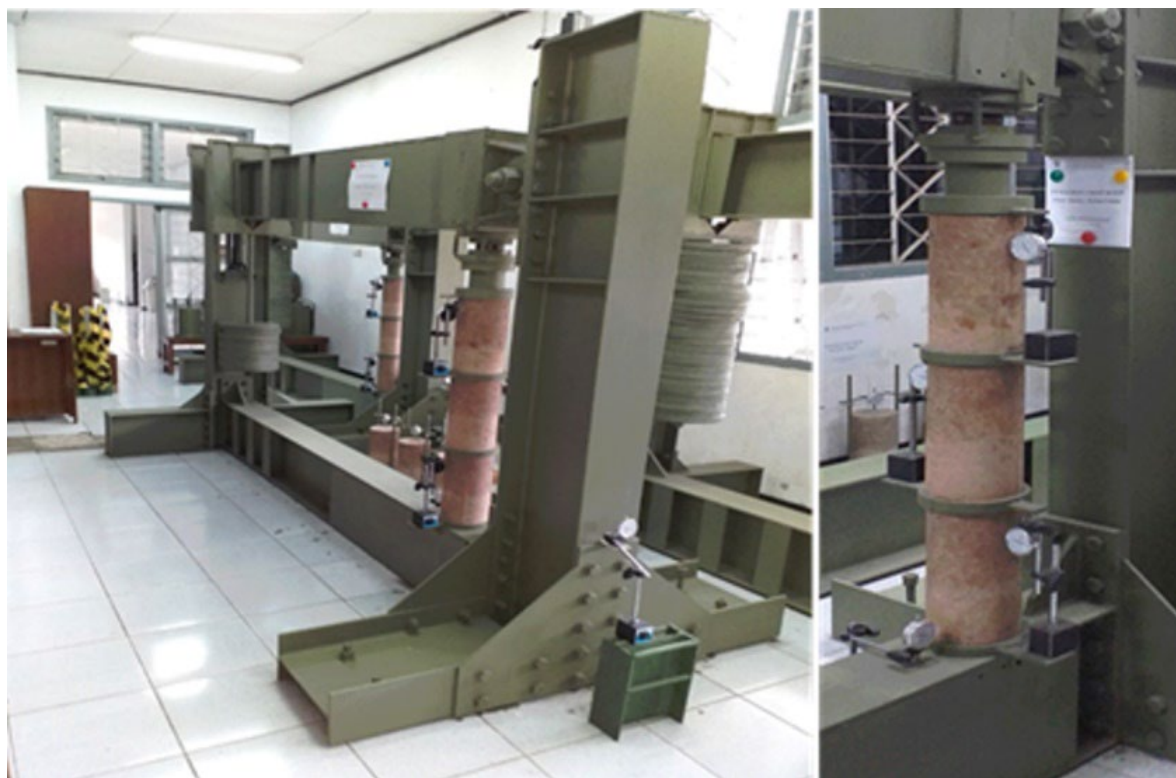
Figure 4. Displacement measurements of concrete creep.
